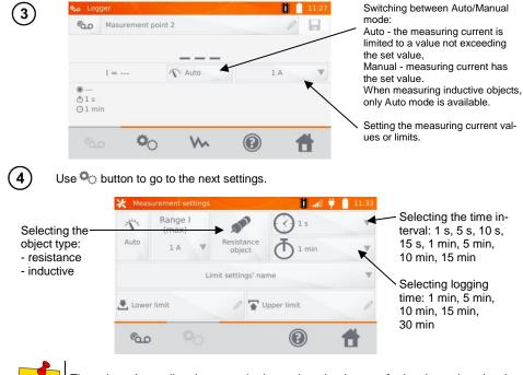
The selected sampling time must be lower than the time set for logging, otherwise the meter will set the default times.
