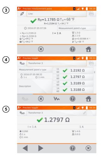
When using the logger, clicking the field with results will cause the meter to display the individual samples. You may scroll them using , buttons. Use button to display the graph.
