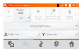
If necessary, select temperature limits from the database (click Limit settings' name) or set the required limits for the performed measurement by clicking Lower limit and/or Upper limit.
