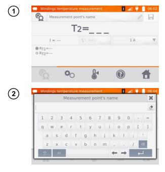
When necessary, name the measuring point.
