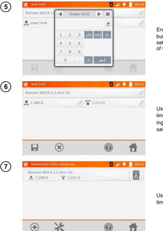
Enter the lower limit. Use button to go to the upper limit setting. You can set only one of the limits.
