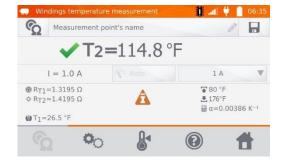
R<sub>T1</sub> – resistance of the cold winding
