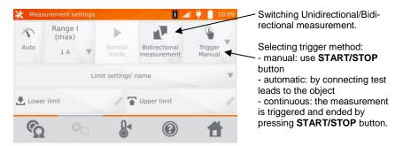
Boxes for setting the range and measurement current on the screen above correspond to the same boxes shown in the previous screen.
