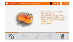
After the desired working time turn off the engine, reconnect the meter to the motor winding and press **START/STOP**.
