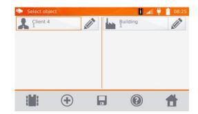
After adding and saving the object (also subobjects according to the needs), click the object and then button - the measuring point with the measurement result will be saved automatically.
